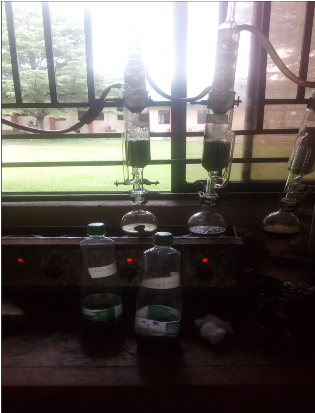
Plate 3. Extraction of plant leaf oils
